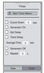
With the original Timer function in v5, we eventually added options to include a countdown before starting the measurement (so the engineer could activate the function and still have time to get into place for the measurement), and the ability to turn on and off the generator (so the engineer is aware of when the measurement has started and has ended).
